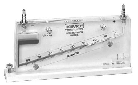
The MT range of inclined liquid column portable manometers, developed and manufactured by KIMO, are particulary recommended for those in the heating trade for checking pressures in chimney flues, combustion chambers, filters...
