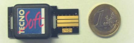
The *TempStick*<sup>®</sup> temperature Data Logger is a miniature temperature sensor: it's a rectangular device measuring 50 X 22 mm and is 10 mm high.
