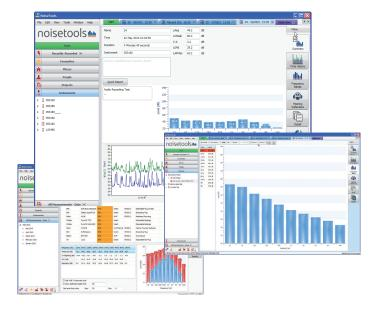
In addition to the noise measurement data, information about the last calibration is also stored. The AuditStore data can be downloaded from the instrument when required, which allows for the measurements to be checked against the AuditStore.
