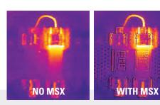
PRODUCE CRISP THERMAL IMAGES See the detail needed to troubleshoot faults and gauge their severity
