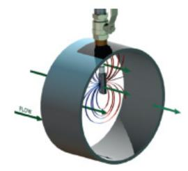
on plastic pipes, the electromagnetic flow meter requires electrical grounding by connection to grounding rings or ground probes inserted into the pipe. Readings are not affected by the fluid temperature, pressure, or viscosity.
