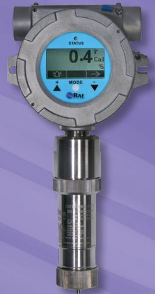
The RAEGuard 2 PID is a fixed photoionization detector (PID) that measures a broad range of volatile organic compounds (VOCs). The RAEGuard 2 PID operates on 10 to 28 VDC and provides an analog (4-20mA) three-wire signal output, and RS-485 Modbus digital signal output. Calibration and maintenance have been greatly simplified as the digital PID module can be easily removed in hazardous locations for calibration or maintenance.
