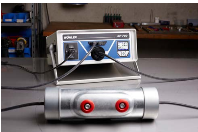
Component test on small, individual components.
